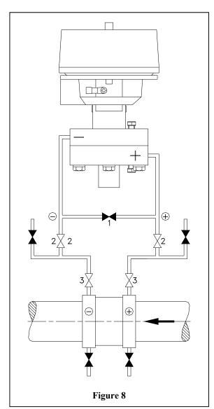
As for differential pressure switches model 3.28, 3.29 3.48 and 3.49, please refer to figure 8 and proceed according to the following instructions:
